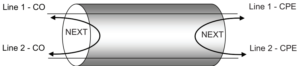
Figure 1: Example of NEXT Interference Between Two Pairs
