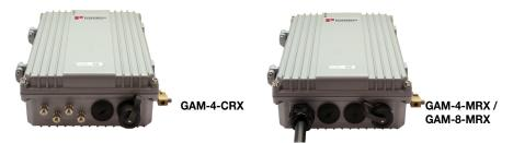
The GAM-4-MRX and GAM-8-MRX respectively have four (4) and eight (8) MIMO ports and support Reverse Power Feed (RPF) from G1001-MR devices, one per G.hn port. The GAM-4-CR has four (4) COAX ports and supports RPF mode from G1001-CR devices, one or more (in Point-to-Multipoint mode) per G.hn port.
