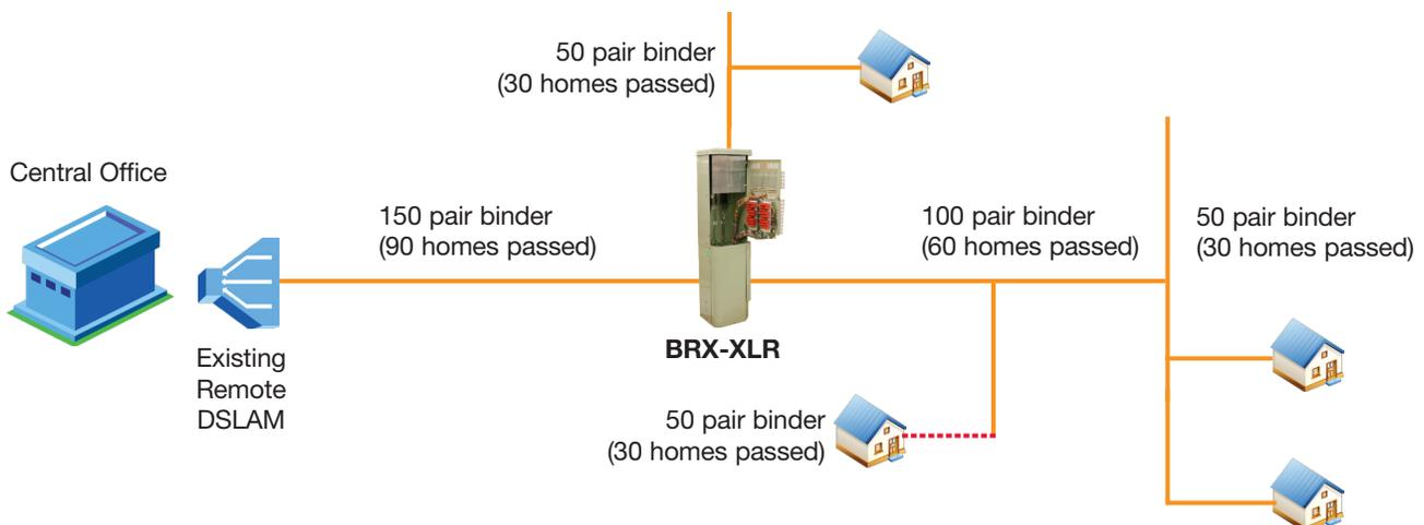
With the BRX-XLR, true broadband services are available significantly deeper into the access network unlocking additional revenues from existing subscribers and from new subscribers as well.
