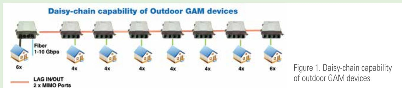
Figure 1. Daisy-chain capability of outdoor GAM devices
