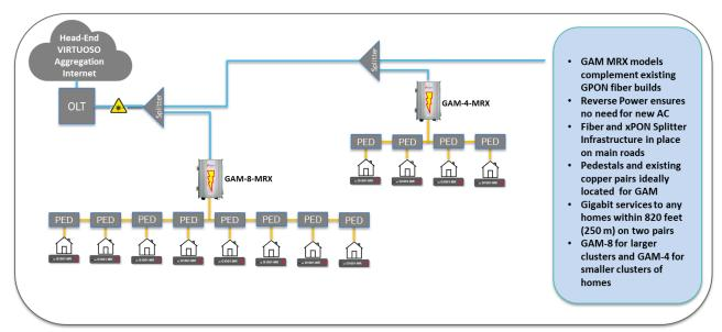
Figure 9: Maximizing low density / rural fiber Gigabit coverage with GAM devices
