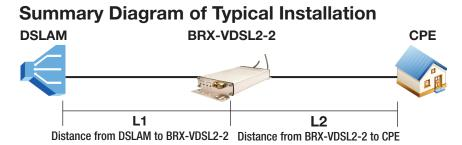
IMPORTANT NOTE: The BRX-VDSL2 unit is powered from the Sealing Current found on a standard POTS pair. Each pair of the BRX-VDSL2-2 is powered independently with each pair requiring the presence of the -48Vdc sealing current for proper operation. The BRX-VDSL2-2 will not operate on a dry pair (line with no -48Vdc sealing current). You can use the Positron BRX Power Injector to provide the -48Vdc sealing current when operating on dry pairs.
