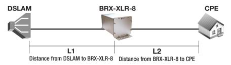
IMPORTANT NOTE: The BRX-XLR unit is powered from the Sealing Current found on a standard POTS pair. Each pair of the BRX-XLR-8 is powered independently with each pair requiring the presence of the -48Vdc sealing current for proper operation. The BRX-XLR-8 will not operate on a dry pair (line with no -48Vdc sealing current). You can use the Positron BRX Power Injector to provide the -48Vdc sealing current when operating on dry pairs.
